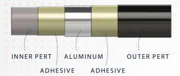
INNER LAYER OF NATURAL PE-RT material has excellent chemical resistance
